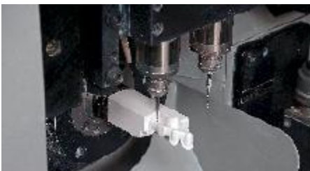
Fig. C The robust Katana milling machine uses the STL files to mill zirconia frameworks to exact details.
